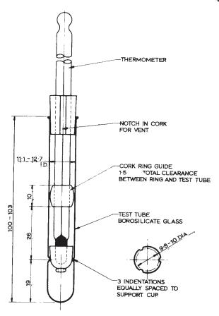
Note 1—Dimensions in millimetres. FIG. 2 Assembled Apparatus
