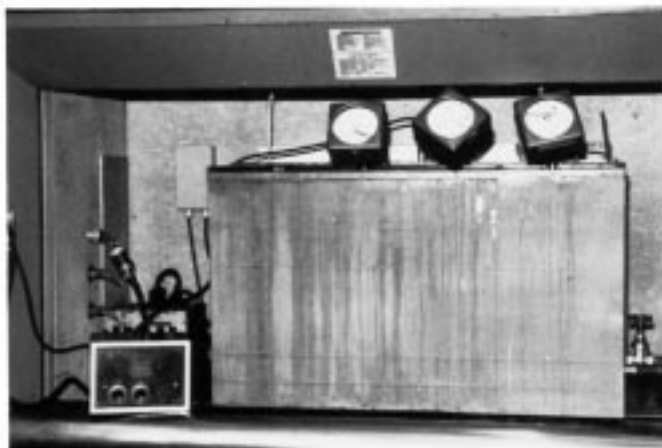
FIG. 1 Rotating Vessel Oxidation Test Apparatus
